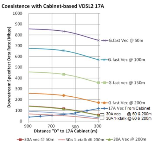
**Figure 6: Comparison of FTTdp Copper Technologies in Same Wire Bundle as FTTN VDSL2**
