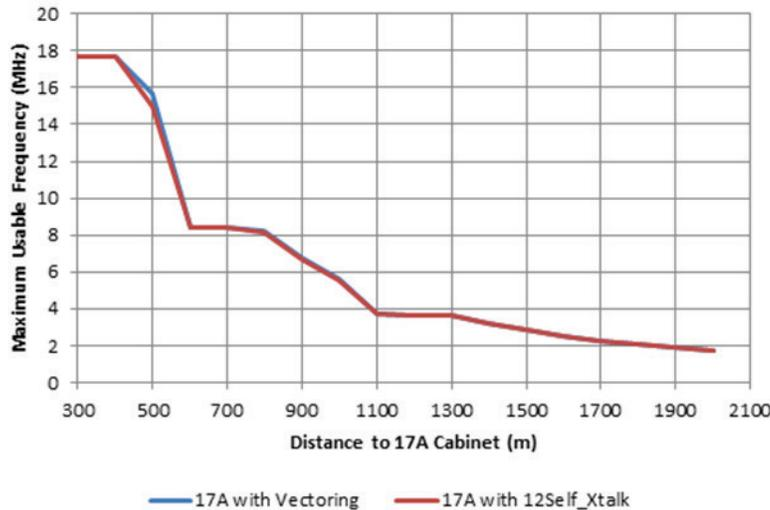
Figure 5: Bandwidth Used by FTTN VDSL2 as a Function of Distance “D”
