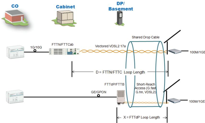
Figure 4: Deployment Scenario of FTTN Mixed With FTTP in the Same Wire Bundle
